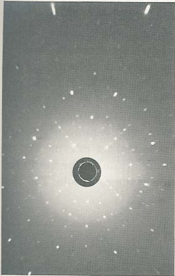
Figure 6 Laue pattern of a silicon crystal in approximately the [100] orientation. Note that the pattern is nearly invariant under a rotation of 2\pi/4 . The invariance follows from the fourfold symmetry of silicon about a [100] axis. The black center is a cut-out in the film. (Courtesy of J. Washburn.)
