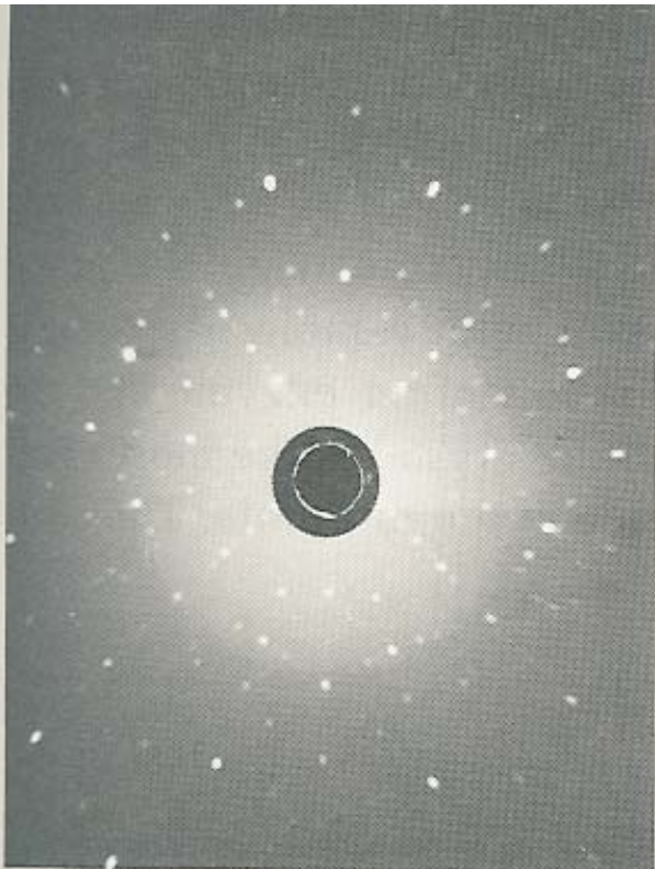
Figure 6 Laue pattern of a silicon crystal in approximately the [100] orientation. Note that the pattern is nearly invariant under a rotation of 2\pi/4 . The invariance follows from the fourfold symmetry of silicon about a [100] axis. The black center is a cut-out in the film. (Courtesy of J. Washburn.)
